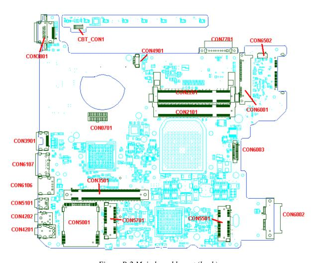
Figure B-2 Main board layout (back)
